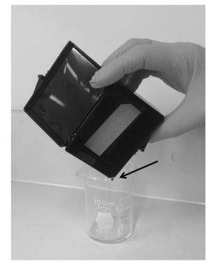
**Fig. 3. Proper decanting technique**. The solution is poured from the incubation box into a beaker while the corner of the box makes contact with the lip of the beaker (arrow). The PIP Strips stay in the bottom of the box without using tweezers to keep it in place. This should be performed quickly but carefully without allowing the blot to dry out. The next solution should be added immediately after decanting.
